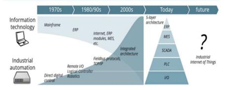
ERP = Enterprise Resource Planning MES = Manufacturing Execution System SCADA = Supervisory Control and Data Acquisition PLC = Programmable Logic Controller I/O = Input/Output signals Source: IoT Analytics
