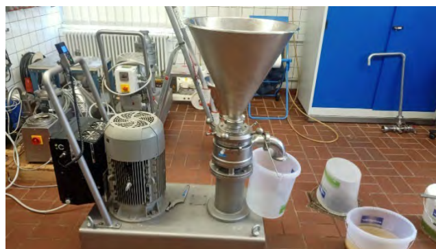
Figure 1 Experimental test on the “colloidal mill type E” of Probst&Class (DE) for resin grinding”
