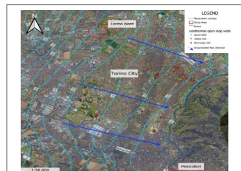
Hydrogeological context of Torino with location of open-loop geothermal plants for feasibility study at two IREN sites Torino Nord and Moncalieri
