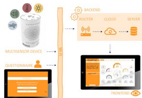
Fig. The PROMET&O system for IEQ monitoring, occupants' feedback on comfort perception collection and data visualization
