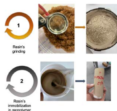
Fig. Fundamentals steps of the new process for the conditioning of IEXs
