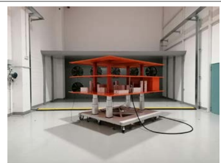
Scaled mockup of an offshore platform inside the test chamber of the SEASTAR WT.
