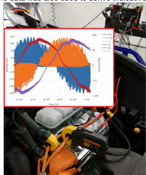
3-phase AC motor power measurement
