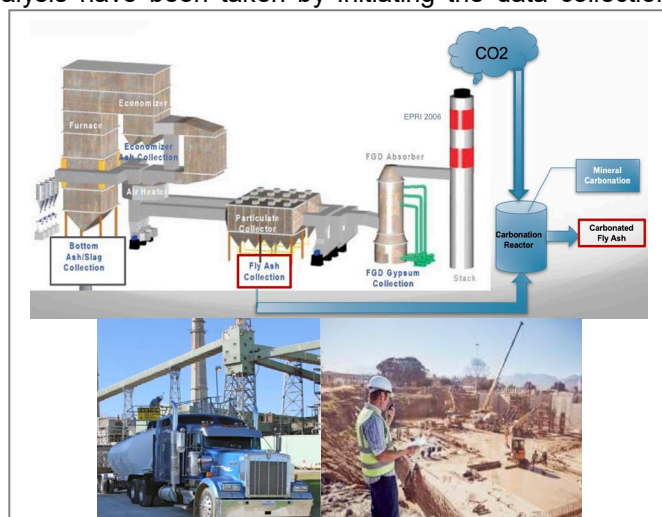
Fig 1. Carbonation process at coal plant, transportation, and use of carbonated fly ash
