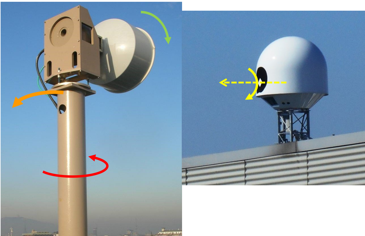
Fig.3: Outdoor test range: the AUT mount (left) and the SRC mount (right).
