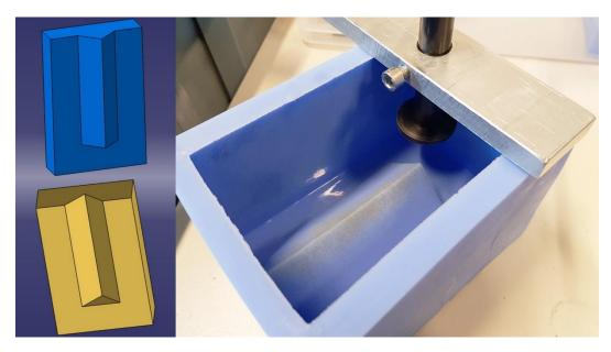
Figure 58 "V-shaped" base mould.
