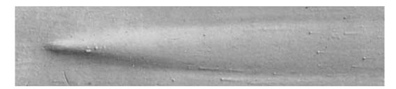
Figure 32 Mould showing a flute at Vt/d = 1.5. Current from left to right. The portion of the bed shown in the photo is 10 cm wide [57].
