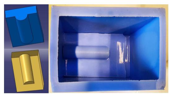
Figure 60 "U-shaped" base mould.
