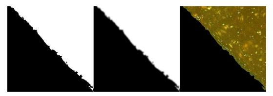
Figure 74 Three main processes (optimised for the lower surface) to detect the body in the photo. On the left: binarization of the photo obtained by the subtraction of the blue channel from the red channel. In the middle: Gaussian filter applied to the previous photo. On the right: Binarization of the photo in the middle and multiplication by the original photo.
