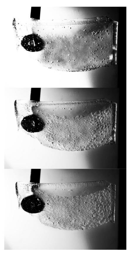
Figure 68 Evolution in time (from top to bottom) of the pattern on a convex surface on a hardcandy block inclined 45° with respect to the horizontal line with no salt added to the aquarium water. Each photo has the same spatial resolution and is taken 30 minutes after the preceding one.
