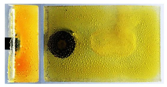
Figure 51 Lateral photo (on the left) and frontal photo (on the right) of the same hard candy block, whose dispersed air bubbles were not removed with the vacuum chamber. The base of the block is 134 mm long and 90 mm width.
