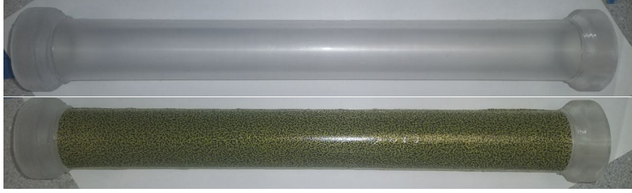
Figure 3.5: Collapsible tube before (top) and after (down) the application of the tattoo paper
