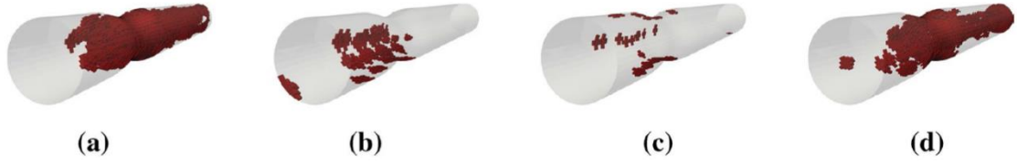
Figure 18: reduced mesh for Navier-Stokes operators of the HROM. The panels represent the cells of the full mesh (red elements) required for the calculation of the coefficients used to impose the interpolation constraints on DEIM (convective, Laplacian, pressure-gradient and pressure-Laplacian operators). The background geometry refers to the mean geometry obtained from the geometric parametrization (transparent background, see Figure 17). [27]
