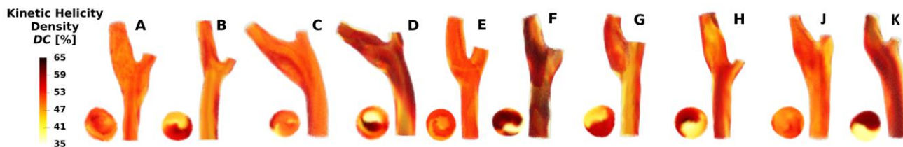
Fig. 11. Volumetric maps of DC for the ten “all-to-all” H_k -based networks. The CCA7 cross-sectional views highlight the existence of two clearly separated low and high DC regions, according to the existence of two distinguishable, counter-rotating, and dynamically correlated helical flow structures.
