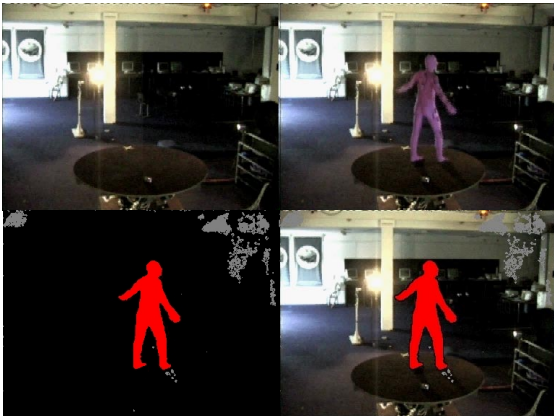
Fig. 5 (a-d): the scene model, a frame of the sequence and the extracted silhouette
